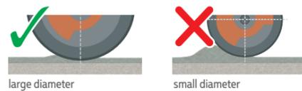
The practice has shown that a larger drum diameter has positive effects on the evenness after the compaction process. This is, among other, proven by the following formula:
